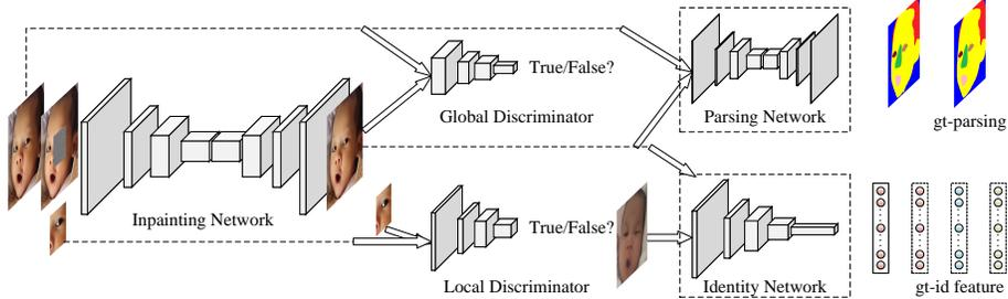
**Fig. 1.** The structure of IP-GANs. They consist of five networks: an inpainting network acting as the generator, two discriminate networks as the discriminator, a parsing network for facial harmony, and an identity network for recovering identity cues.
